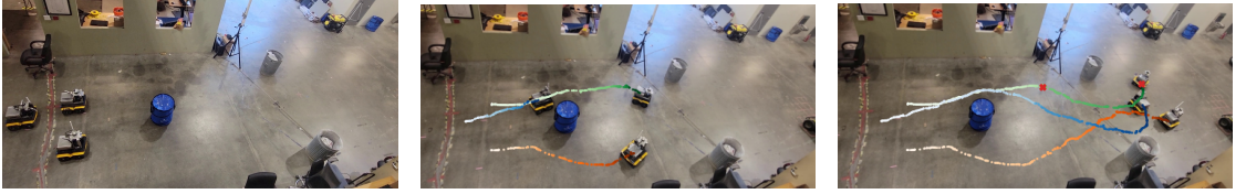
Figure 7.8: Snapshots of the hardware experiment with color coded trajectories for the different robots. The intensity of the color increases with time. In the last snapshot, the red x's indicate the two different waypoints for the leader of the team. The environment has dimensions 4\text{m} \times 9\text{m} .
